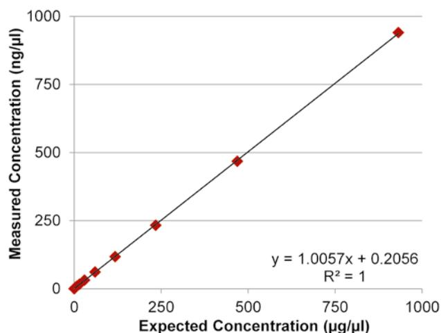
Figure 2: Samples (mean value) in the range of 1.89 – 932 ng/μl were measured with path length 0.67 mm.
